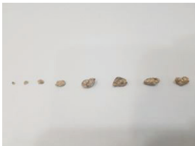
Figure 1: Weathered granite stones of various size with rough surfaces
